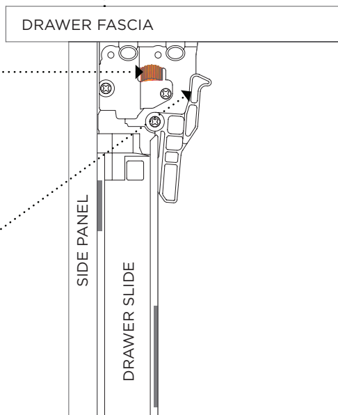
BOTTOM VIEW OF DRAWER: DRAWER SLIDE FUNCTIONS
